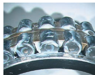
Photo. 6.2 Filling grease into cylindrical roller bearing
